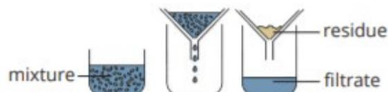
This method is used to separate an **insoluble solid** from a **liquid**. The solution is passed through a filter paper and a funnel.
